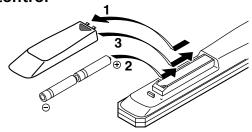
Remove the battery compartment cover.
